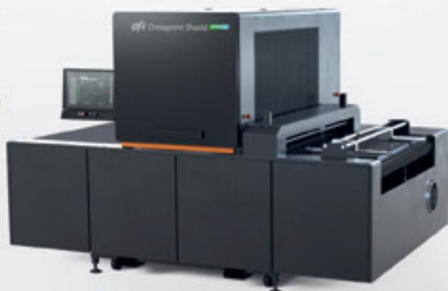
EFI Cretaprint Shield, equipped with up to 2 printing bars, can be used for digital glazing and other ceramic applications to do the full-digital decoration. Complement your current equipment by placing EFI Cretaprint Shield prior to tile printing to apply digital glaze or post-tile decoration to apply glues and other effects.
